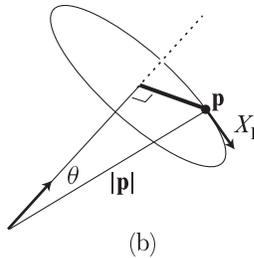
radius  $|\mathbf{p}|$ , and  $X_{\mathbf{p}}$  has length  $|\mathbf{p}| \cdot |\mathbf{w}|$ . More generally (b), the point  $\mathbf{p}$  rotates in a circle of radius  $|\mathbf{p}| \cdot |\mathbf{w}| \cdot \sin \theta$ , where  $\theta$  is the angle between  $\mathbf{w}$  and  $\mathbf{p}$ . Thus,  $X_{\mathbf{p}}$  is just the geometrically defined cross-product  $\mathbf{p} \times \mathbf{w}$ .
