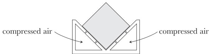
side view of a block sliding on an air trough
