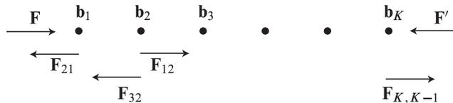
exerted on  $\mathbf{b}_1$  by  $\mathbf{b}_2$ , requiring an equal but opposite force  $\mathbf{F}_{12}$  on  $\mathbf{b}_2$ , which would in turn be balanced by a force  $\mathbf{F}_{32}$  exerted on  $\mathbf{b}_2$  by  $\mathbf{b}_3, \dots$ , leading finally to a force  $\mathbf{F}_{K,K-1}$  exerted on  $\mathbf{b}_K$  by  $\mathbf{b}_{K-1}$  that balances  $\mathbf{F}'$ .
