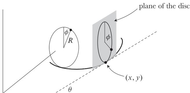
coordinates  $(x, y)$  of the point at which the disc rests on the plane, the angle  $\phi$  that a fixed point on the disc makes with the vertical, and the angle  $\theta$  that the plane of the disc makes with the  $x$ -axis.
