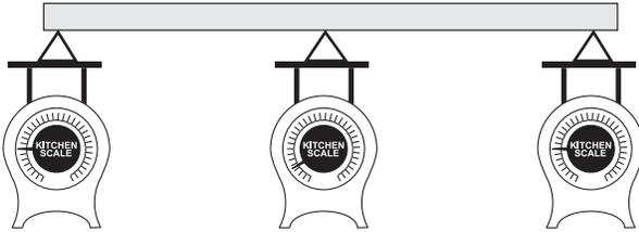
confidently expecting the middle scale to register over 3 times the readings of the end scales. But, as I discovered, and showed at the lecture, the end scales actually registered much larger weights than the middle scale!
