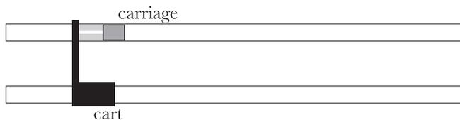
the cart must be given the acceleration  $\alpha_1 = 2a_1$  in order for the two springs to be compressed simultaneously to the length  $L_0$ . Although this might seem clear if you think in terms of the usual  $\mathbf{F} = m\mathbf{a}$  law, it is basically an experimental fact that we have to test, along with similar tests for three springs, four springs, etc.
