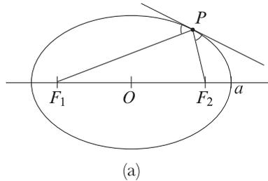
has the “focal point” property that a light ray starting from  $F_1$  passes through  $F_2$ , i.e., that the two angles indicated in (a) are equal.
