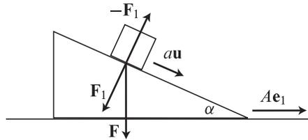
our inertial system. Note that in our picture, we actually have  $A < 0$ , so that the arrow  $A\mathbf{e}_1$  points in the opposite direction, since the force  $\mathbf{F}_1$  causes the block to slide to the left.
