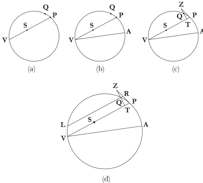
$VA$ , and then (c) we draw the line  $TQ$  perpendicular to  $SP$ , and extend it until meets the tangent line to the circle at  $P$  in the point  $Z$ . Finally, (d) we draw the line  $LR$  parallel to  $VP$  intersecting the circle at  $L$  and the tangent line at  $R$ .
