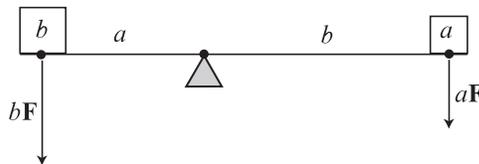
connections between the fulcrum and the earth, but it seems reasonable simply to regard this connection as a mechanism that automatically supplies the proper *upward* force to the fulcrum when the downward forces are applied at the ends of the lever.
