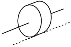
theorem then allows us to compute the moment of inertia around a parallel axis that goes through the edge, a result that we will mention in the next lecture.
