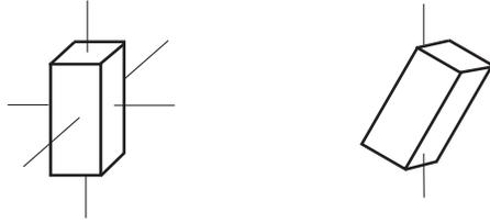
symmetry. You might naively expect that if it were provided with the right initial push it could also rotate about any other axis that passes through the center of mass of the block, as illustrated in the right hand part of the figure, but a little thought should be able to convince you otherwise (note that the angular momentum vector won't be constant).
