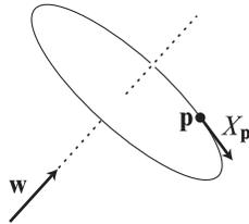
To compute  $X_{\mathbf{p}}$  geometrically, we note that  $X_{\mathbf{p}}$  is clearly perpendicular to both  $\mathbf{p}$  and  $\mathbf{w}$ . Its length is also easy to determine. When  $\mathbf{p}$  happens to lie in the plane perpendicular to  $\mathbf{w}$ , as in (a), the point  $\mathbf{p}$  rotates in a circle of
