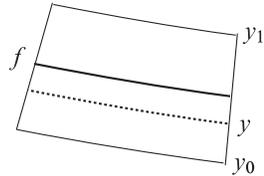
graph of  $f$ , the cross-section of the neutral plane, the dotted line indicates the cross-section of a surface where the stress has the constant value  $y$ . The whole region is filled up by such surfaces having values in some interval  $(y_0, y_1)$ .
