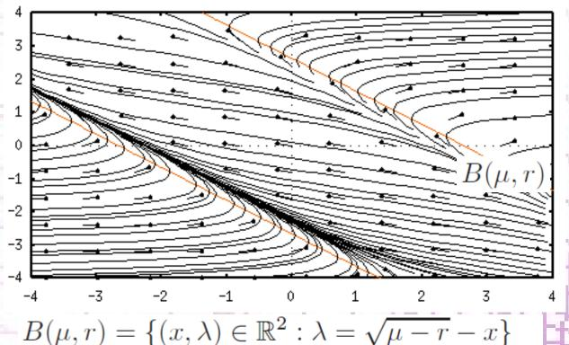
• B( $\mu$ , r) defines a tipping *threshold*. Initial conditions below B( $\mu$ , r) converge to a parallel line, whereas initial conditions above B( $\mu$ , r) have solutions x(t)  $\rightarrow \infty$  as t  $\rightarrow \infty$ .
